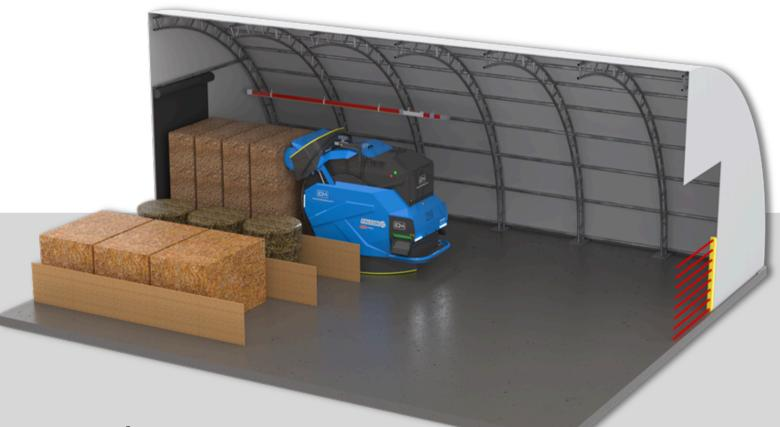
Thanks to the FiberCut system and arms, mixing time is very short, especially if the feed ingredients are pre-cut, by a forage trailer or forage harvester.
